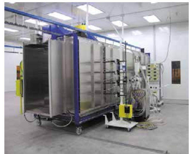
Custom designed booth openings such as operator shields and touch-up windows create a safe and efficient working environment.
