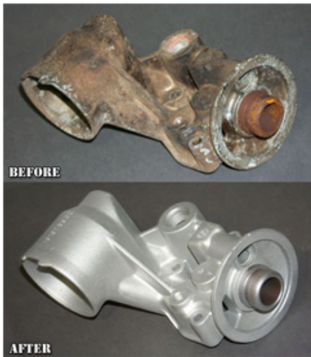
Glass bead blasted component
